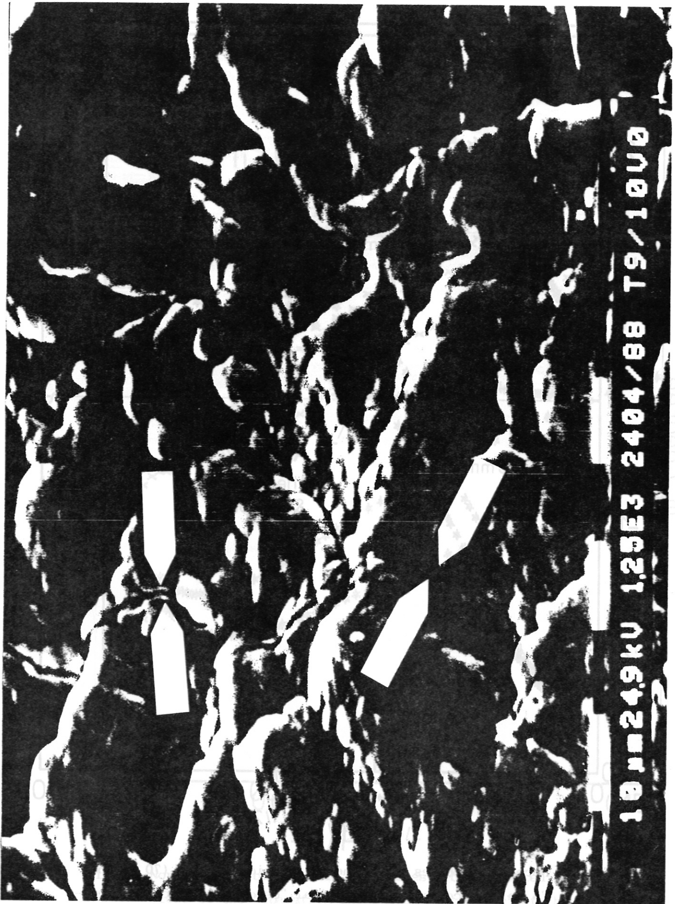
Fig. 9. Electron micrograph from the "inversion" region, showing cracks of approximately 1 \mu\text{m} width in the deposited material.
